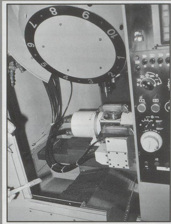
Some of the jobs have to be done by machine. The drilling of the very small holes for things like handrails and radio antenna are so critical, only a machine can do them accurately enough. The people at HAG had to redesign this machine to drill at far higher speeds than normal, in order to achieve greater accuracy and extend the life of the very small drills used.
