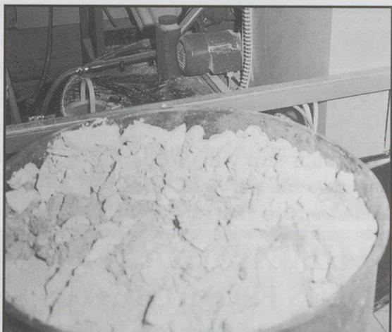
*What looks like clay here, is actually metal dust. As HAG's metal bodies are drilled, reamed and polished, the very fine dust is sucked away at the sites and transported here by ducts. The metal is filtered out and solidified, to be sold off for use in other manufacturing.*
