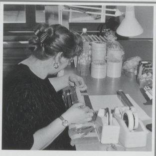
For the other coats of paint, masking off is done by hand: a consequence of the relatively small numbers produced by firms like HAG. It would be far too expensive to set up a machine to do something like this for anything less than 10000 items at a time. Figures like that are only achieved by firms like Märklin or Bachmann.
