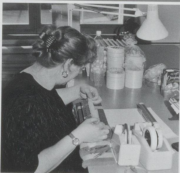
*For the other coats of paint, masking off is done by hand: a consequence of the relatively small numbers produced by firms like HAG. It would be far too expensive to set up a machine to do something like this for anything less than 10000 items at a time. Figures like that are only achieved by firms like Märklin or Bachmann.*
