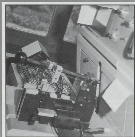
The rotors of the motors are tested for absolute balance, another quality point. Not many other manufacturers bother about this, preferring to install 50p motors in £100 engines.
