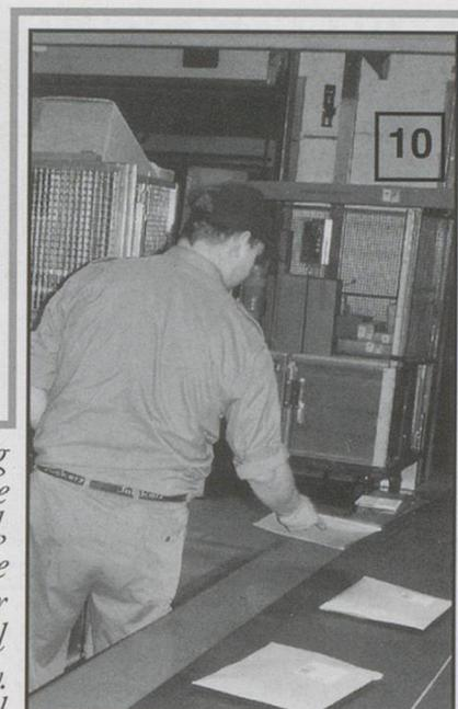
One of the few humans working in the centre. First he has to take out parcels which are oversized, wrongly packaged (i.e. with loose strings that can get caught), or have no bar code. These will have to be handled separately. The others have to be placed with the bar code the right way up on the conveyor belt.
