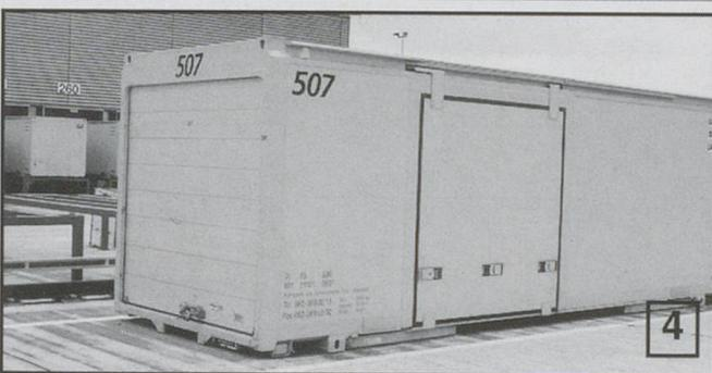
The special swap-bodies (as they cannot be stacked, they are not classified as containers) are built by Frech Hoch in Sissach. They are 24ft. 5in. long, 8 ft. 4 in. wide and 8 ft. 9 in. high. They are in the process of being fitted with a transponder, which will enable GPS tracing of the yellow swap-body. See drawing No. 2 .
