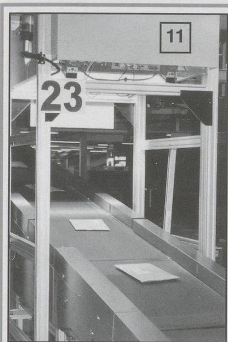
After the bar code has been read by one of these gates, the parcel will be conveyed with full automation. The centre can handle a maximum of 15,000 parcels an hour. These almost flat packets are parcels: the centre does not handle letters.
