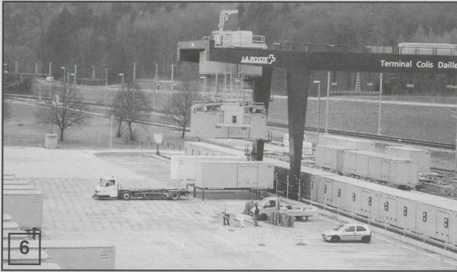
*It is just a short distance to the loading bays at the terminal. A purpose built truck drives under the carrier-bed, connects with the swap-body and the carrier, lifts it off the ground and drives to the correct bay. Here the combination of swap-body and carrier-bed is put back on the ground.*
