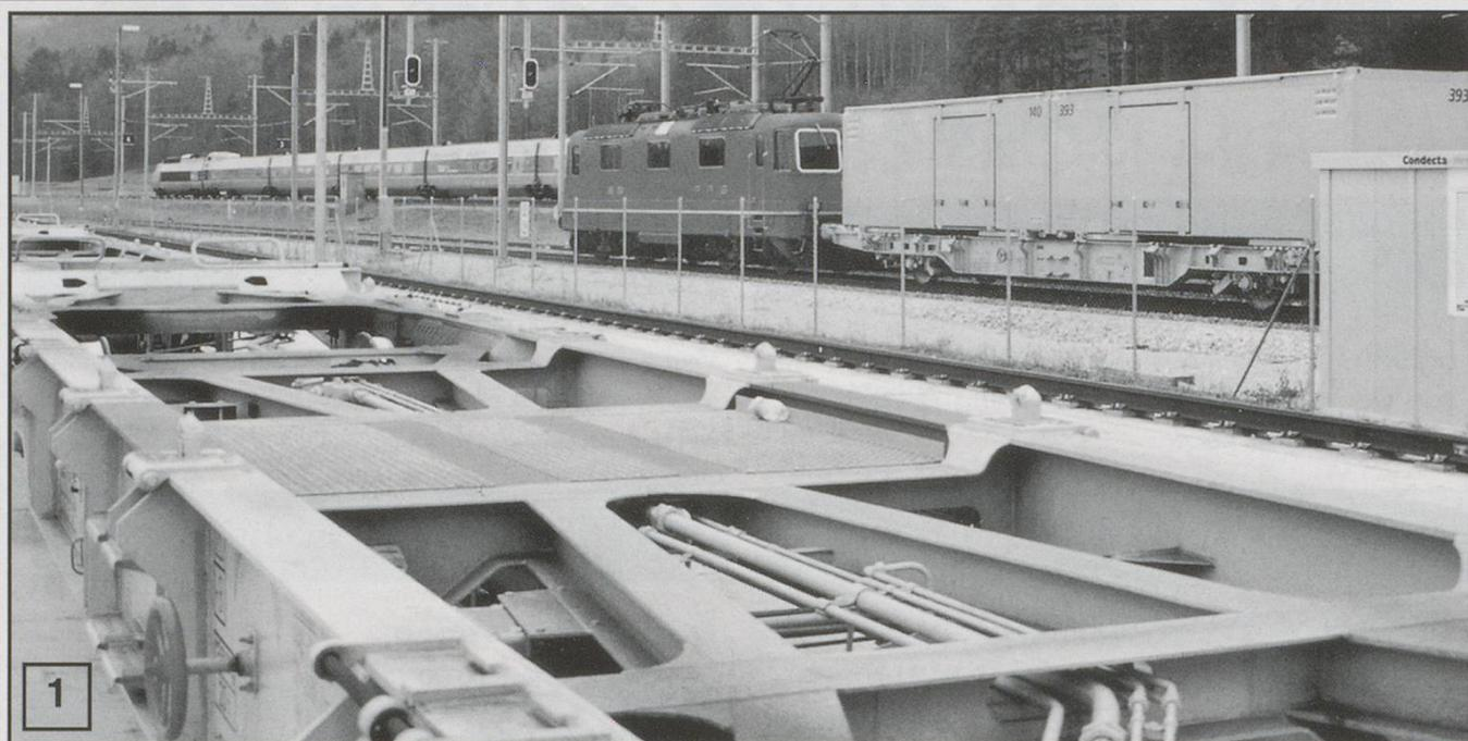
*The TGV racing in the background on its way from Lausanne to Paris, is just about to negotiate the turnoff for Vallorbe. The Re 4/4<sup>II</sup> with its postal train is not quite as fast, but the special two-axle swap-body carrier wagons are capable of running at 75 mph.*
