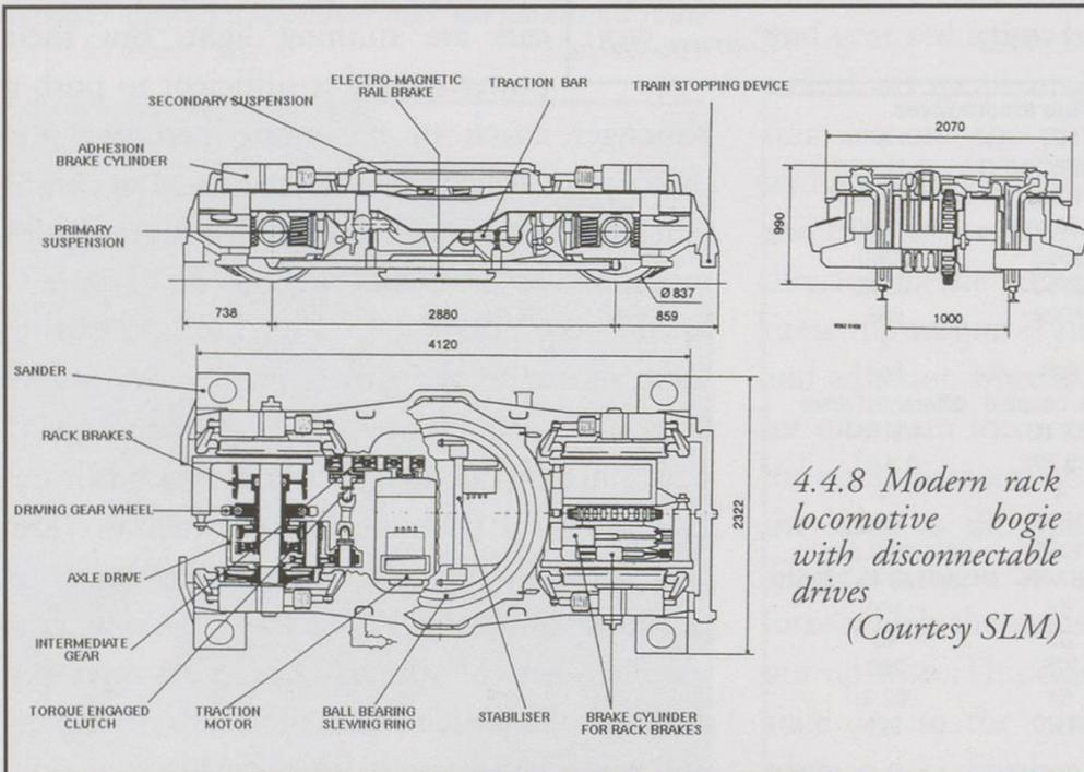
4.4.8 Modern rack locomotive bogie with disconnectable drives (Courtesy SLM)
