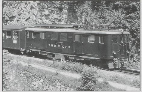
4.4.10 Brünig motor car with two adhesion bogies and one rack bogie descending to Meiringen, August 5th1974. Photo: Hauser
