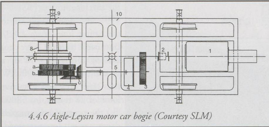
4.4.6 Aigle-Leysin motor car bogie (Courtesy SLM)
