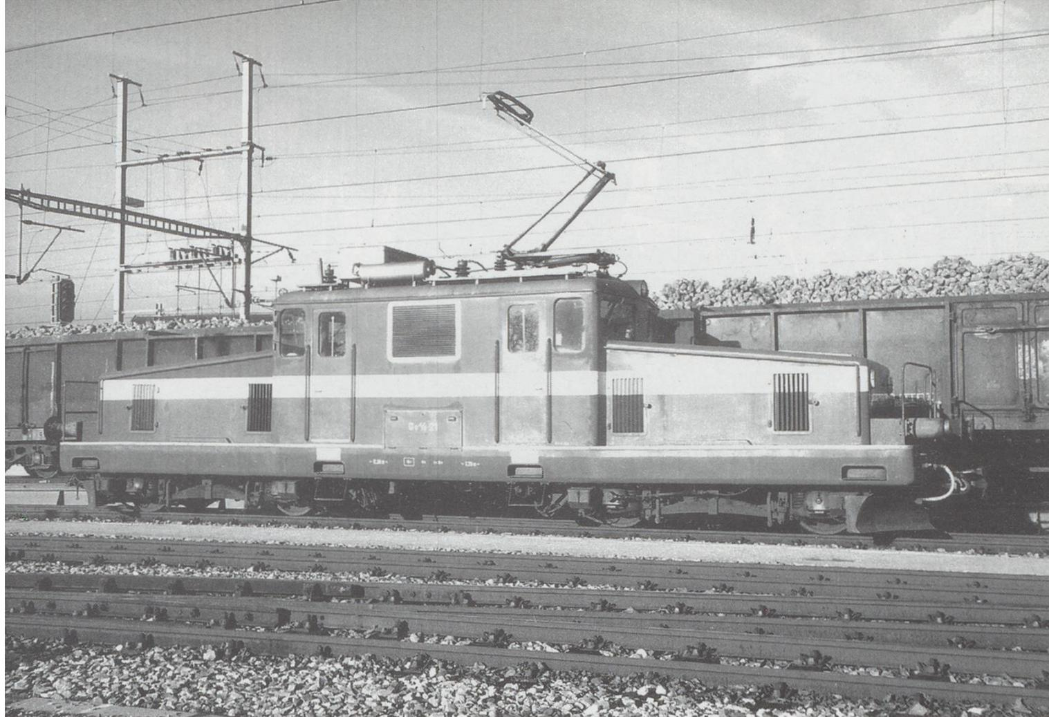
create one vehicle which is now numbered Be4/4 5. In 1950 an electric freight locomotive, Te4/4 21 (now Ge4/4), was constructed in the company's own workshops using parts supplied by SIG and BBC. This is still in service and carries a blue "crocodile" livery.
