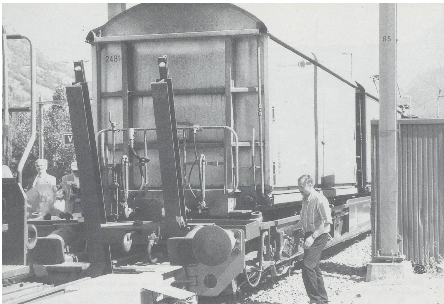
Above: The rails/ramps are raised and lowered hydraulically. The wagon is ready for movement. Below: The standard gauge wagon makes its way to the warehouse propelled by the station tractor.
