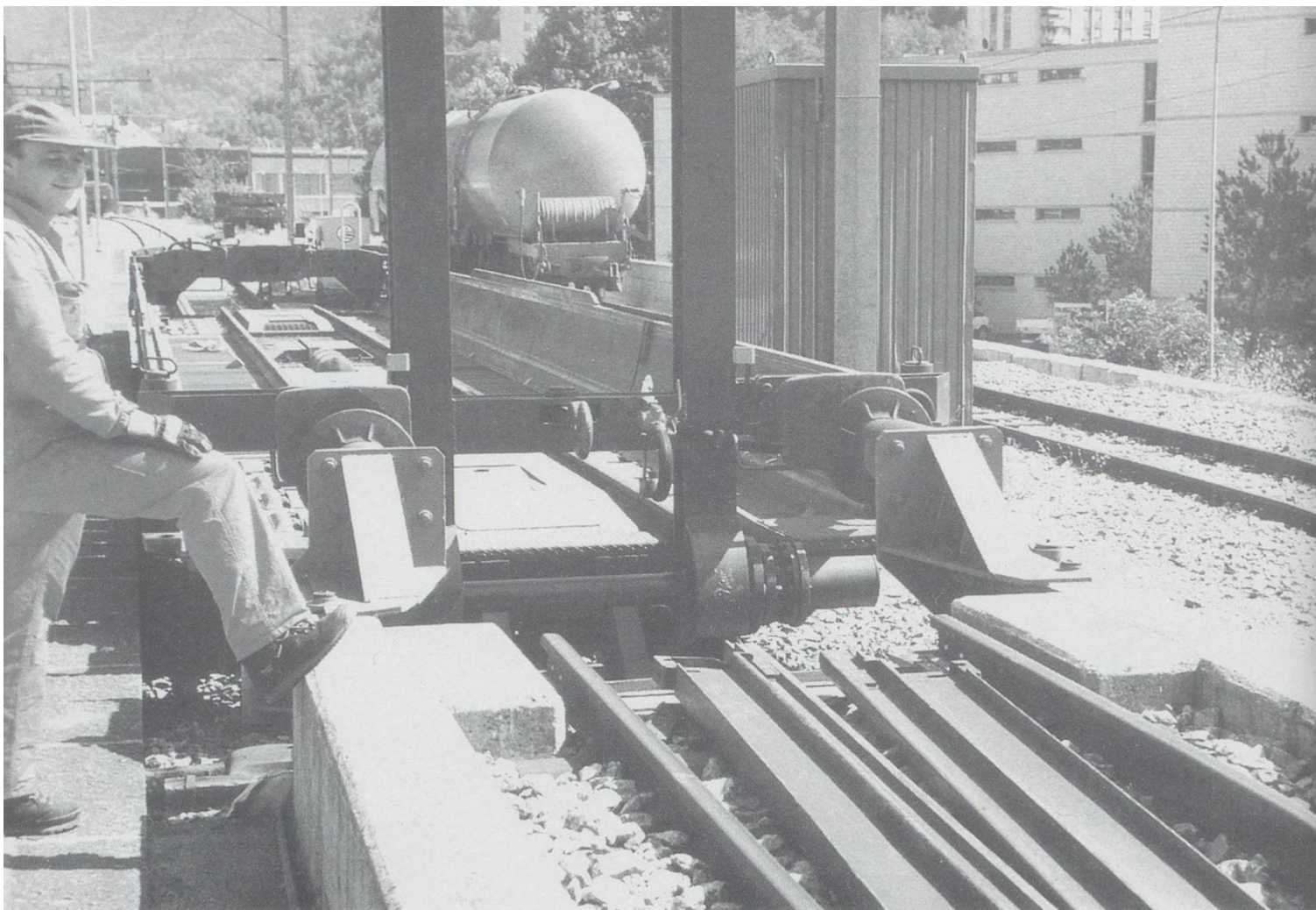
Above: The standard gauge wagon parked at the metre gauge loading dock. Note the buffer beams swing out for loading, then the rail/ramps are lowered. Below: The metre gauge shunter pushes the metre wagons onto the standard gauge wagon. Note the position of the buffers. Photo: Les Heath
