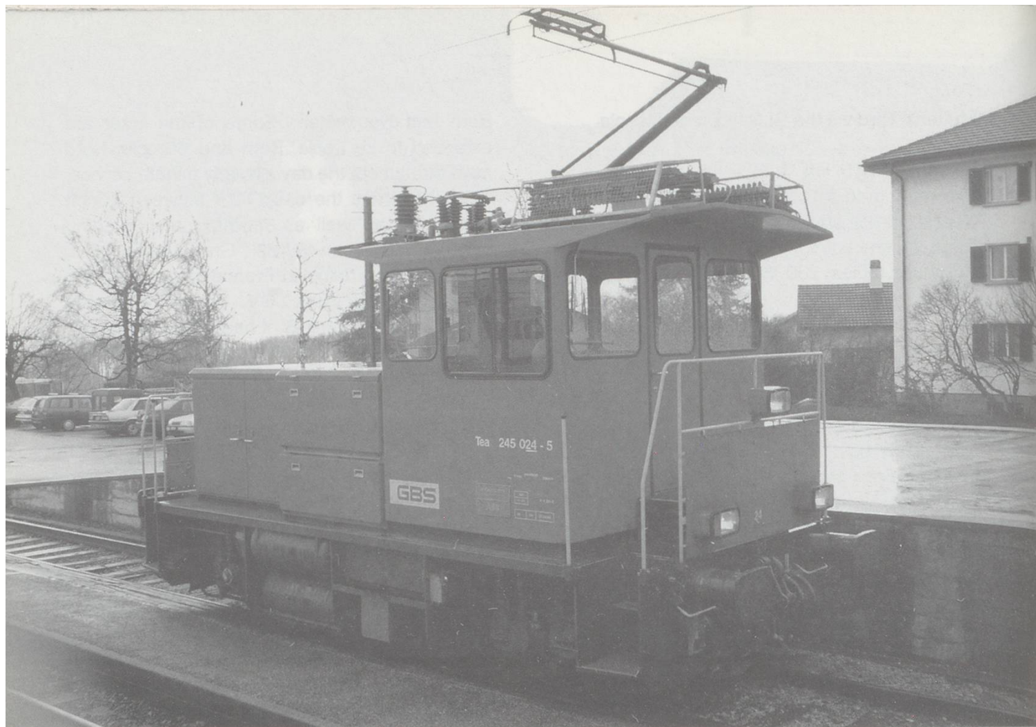
Above: One of the GBS shunters, Tea 245 042, unusual in that it is overhead or battery powered.
