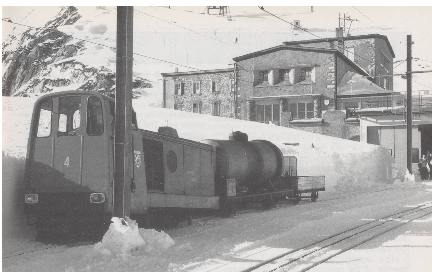
Above: The ex Brienz Rothorn diesel seen here at the summit of Rochers de Naye with a service train taking water to the restaurant, now Hm2/2 4 of the Montreux-Terriet-Glion-Rochers de Naye (MTGN) 6th December 1996.
