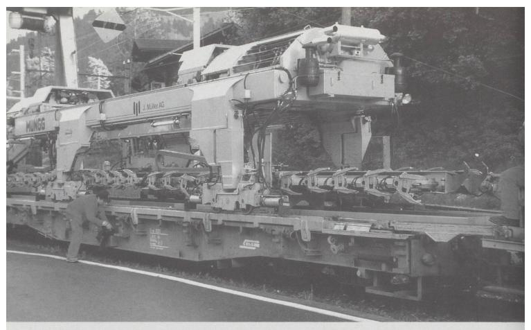
Above: The crane with the lifting spar the fork arms swivel down to pick up the new sleepers. Below: An old section of track being lifted, the new replacement rail can been seen next to the ballast waiting lifting onto the new sleepers. The lifting spar is suspended between the tracked crane and the wagon mounted crane. Note the new sleeper on the left having been dropped with the previous section.
