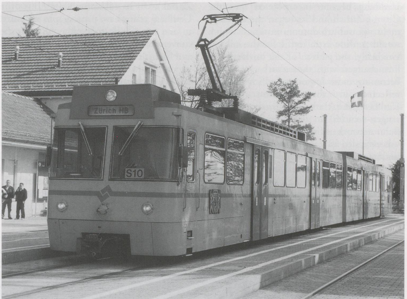
SZU 32 prepares to leave Uetliberg for Zürich HB at 1738 on Tuesday 5/5/98. Notice in particular the offset pantographs.
