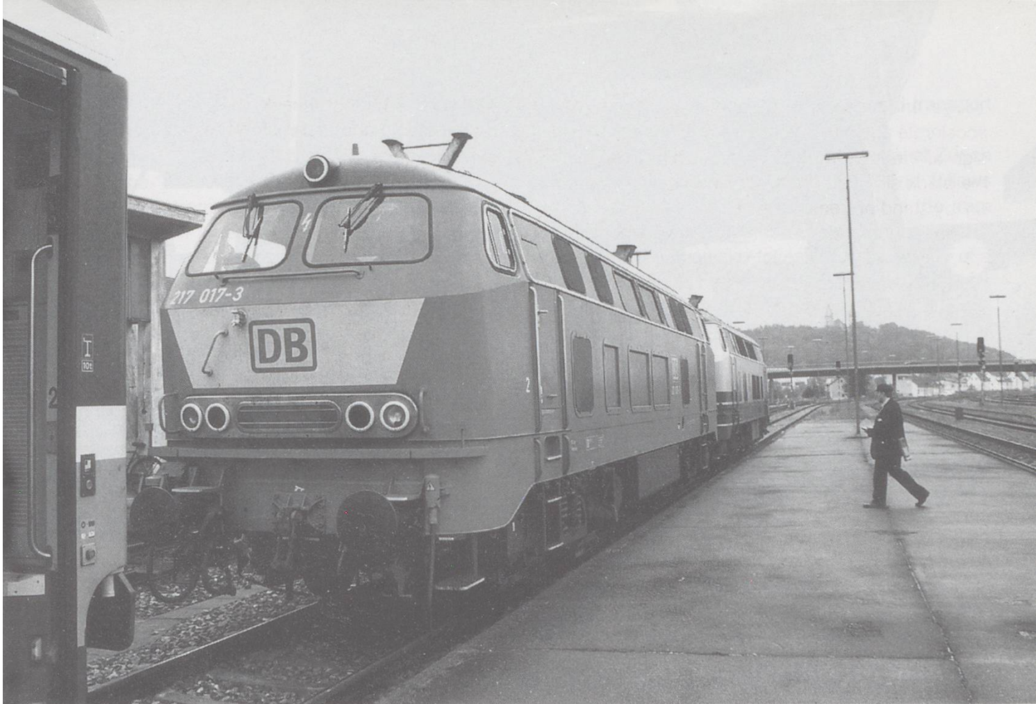
Above: 217 017-3 + 218 215-2 backing onto "Albert Einstein" at Schwandorf, 11.51, 9/10/98. Note the exhaust stacks to avoid damage when running under wires Below: VT09 at Cham, Regental Bahnbetrieb GmbH
