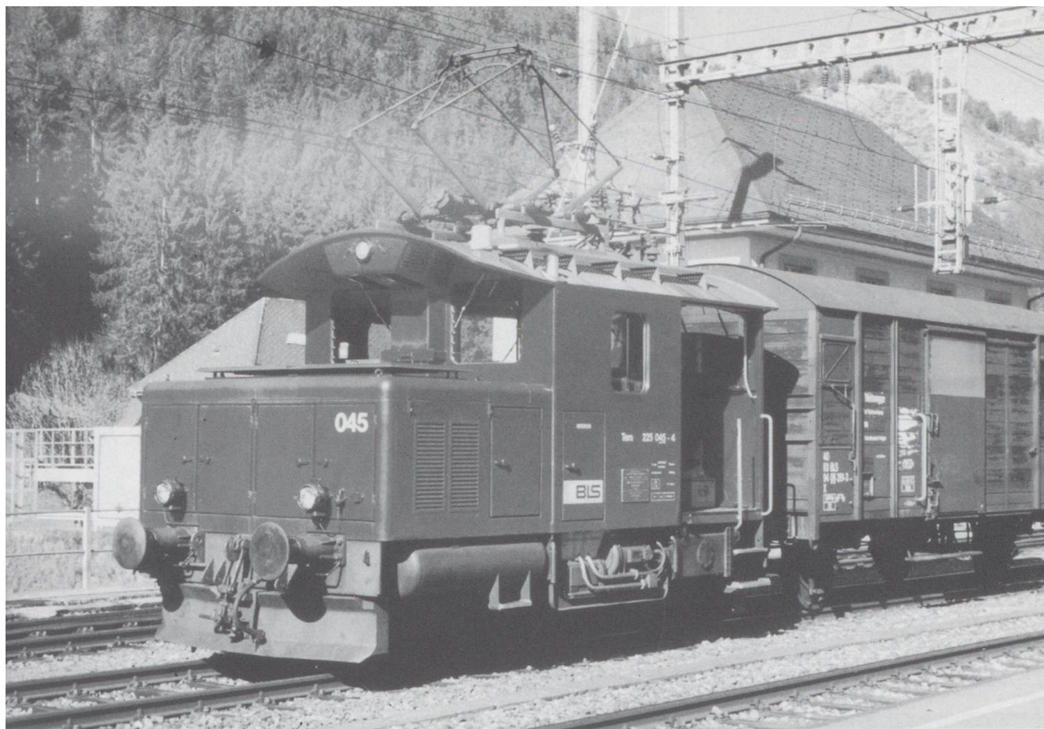
Above: Tem 045 with the point washing train referred to in the article, 30/10/97.
