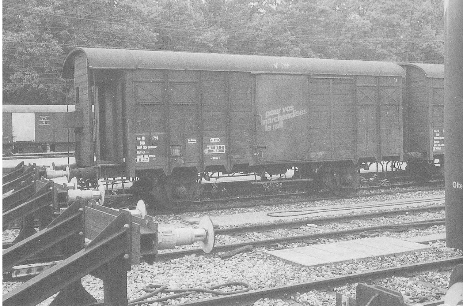
Above: This K3 is now a station stores van at Bülach. The doors of the brakemans cabin have been removed and the old inscriptions painted out on the body, but it retains the door slogan. The new inscriptions forbid the vehicle to leave Bülach station.
