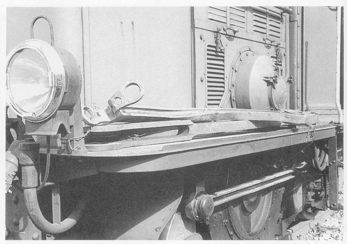
In September 1993 No 413 sheared a crankpin and bent the side rod so thoroughly that it was impossible to straighten it. Replacement was out of the question, not merely on ground of cost but the difficulty of getting a rod forged and machined nowadays. As the remaing four machines were sufficient for the rostered services, 413 was towed to Landquart to supply spares for the balance of the class.
