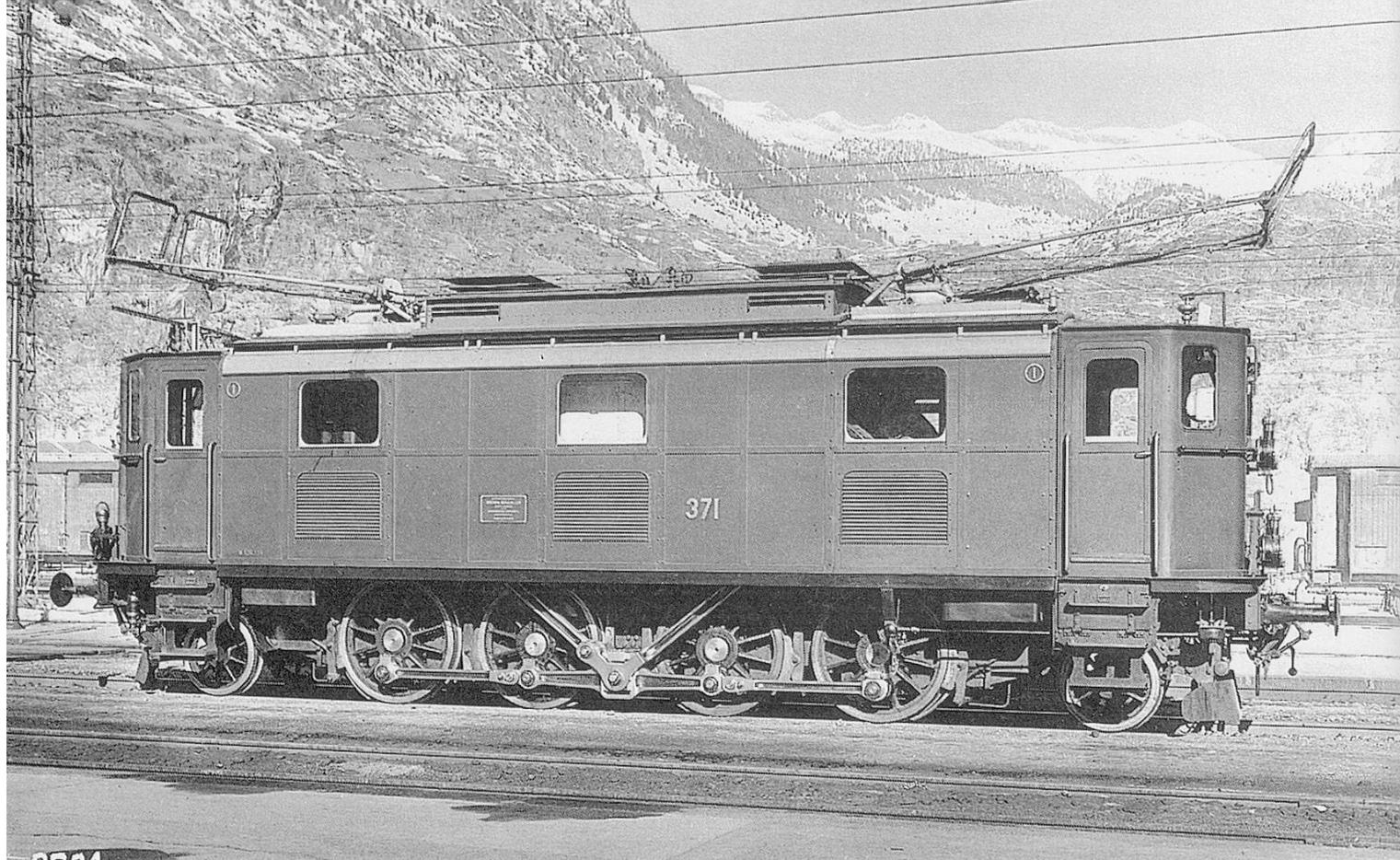
The last new design of the 3-phase locomotives to be built was the Fb4/6 No.371 delivered in 1914. Notice the body style, which is very similar to the SBB Ae3/5, Ae3/6<sup>II</sup> and Ae3/6<sup>III</sup> of the '20s, and also the RhB Ge4/6, built in 1913/14.
