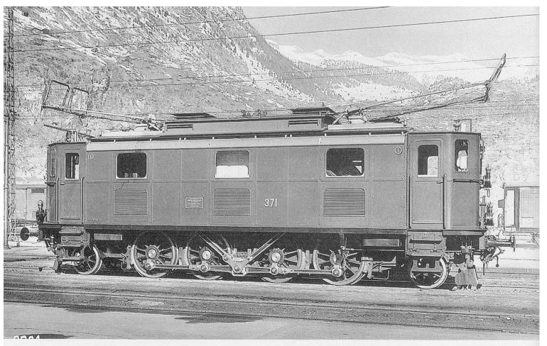
The last new design of the 3-phase locomotives to be built was the Fb4/6 No.371 delivered in 1914. Notice the body style, which is very similar to the SBB Ae3/5, Ae3/6<sup>II</sup> and Ae3/6<sup>III</sup> of the '20s, and also the RhB Ge4/6, built in 1913/14.
