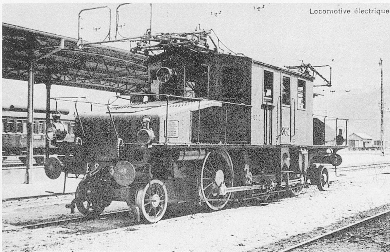
Fb3/5 No.362, one of the locomotives built by Ganz, Budapest, which were hired to the SBB by the FS for a short time. It is fitted with BBC current collectors.
