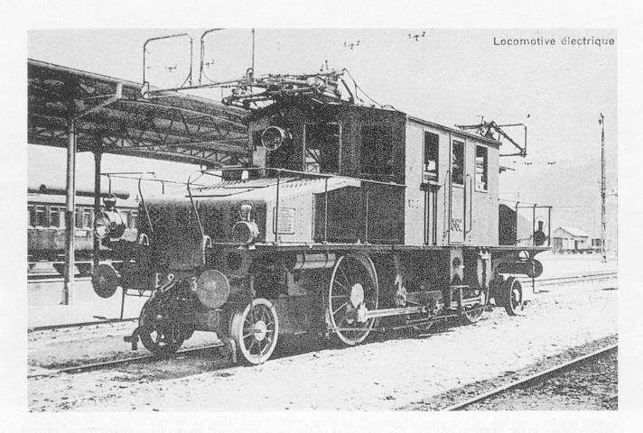
Fb3/5 No.362, one of the locomotives built by Ganz, Budapest, which were hired to the SBB by the FS for a short time. It is fitted with BBC current collectors.
