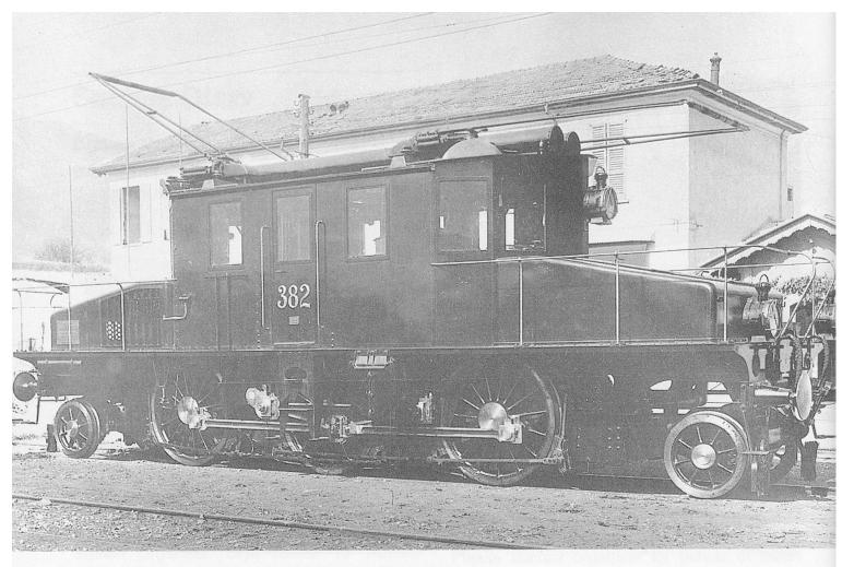
Corresponding to the Simplon N0.362, FS No.382 is of the same type, and shows the simple type of current collector fitted to the Ganz locomotives.
