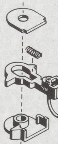
The couplings are not brilliant at coupling on curves if they are mounted on the body of a vehicle, especially at the transition of straight and curved track, because of the lateral off-set of the coupling. (They can, and should, be mounted on the bogies of long bogie stock not fitted with the NEM box and KKK.)
