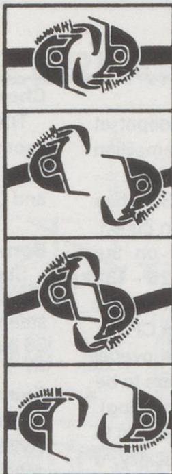
1. Stopped over Delayed-Magnetic Uncoupler, knuckles have opened. "Uncoupled" position.
