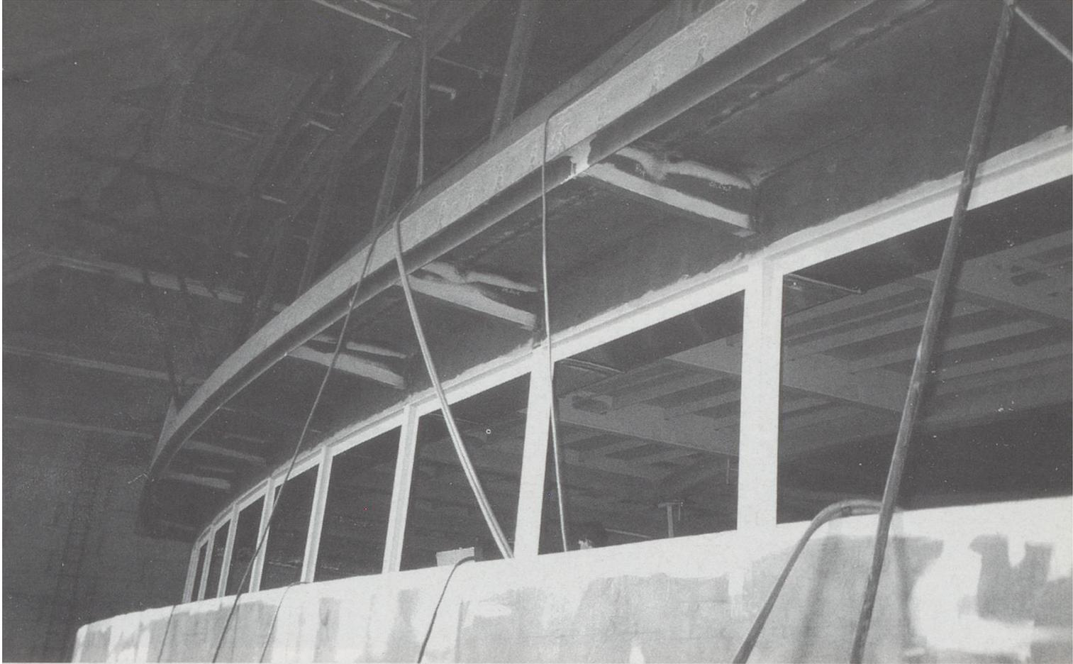
*Above:* Superstructure in place, red primer coat and first white undercoat is evident.
