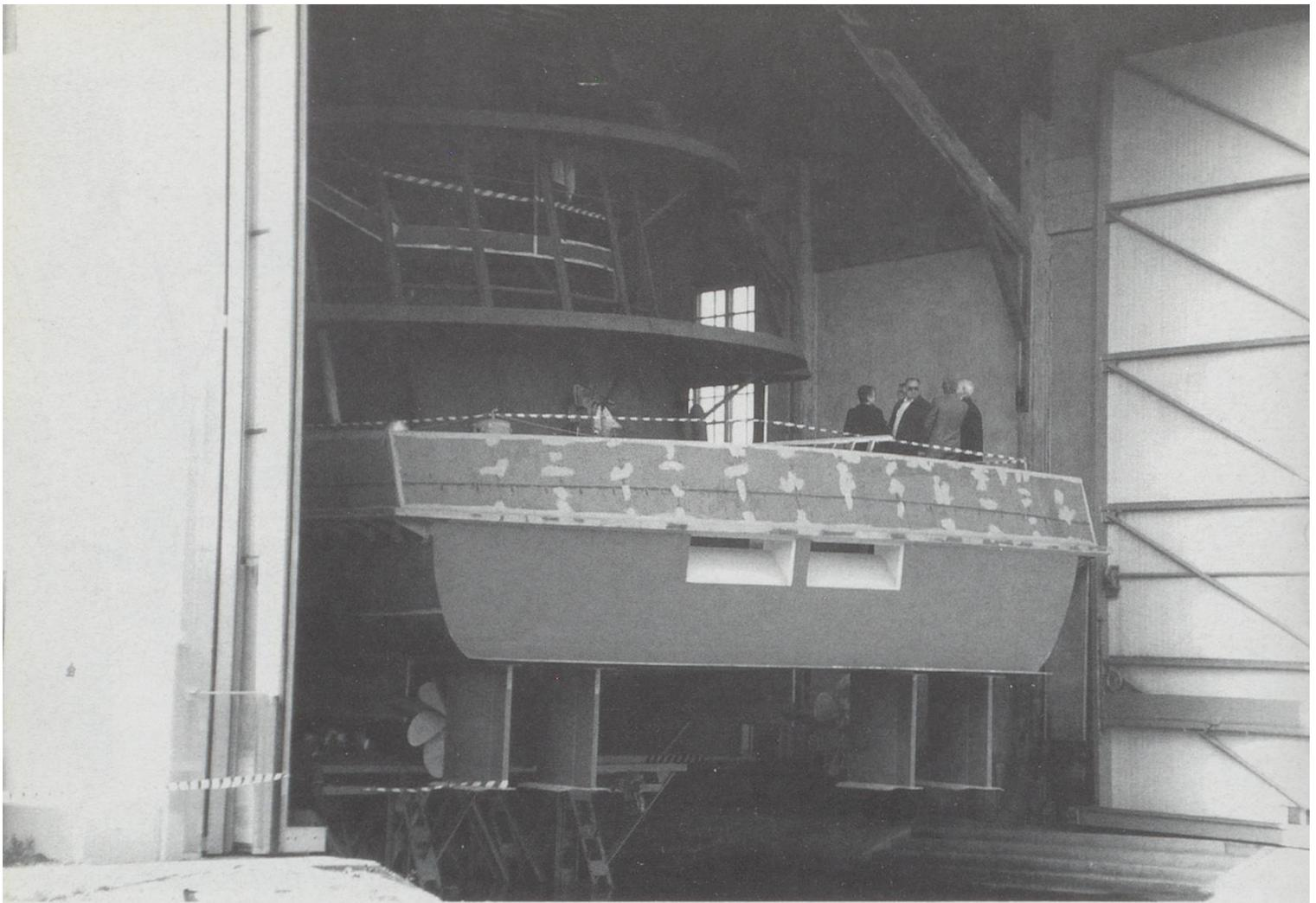
Above: Slightly too long for the shed, the stern protrudes through the doors. Twin screws and four skogs are clearly shown in this shot as well as the aft superstructure.
