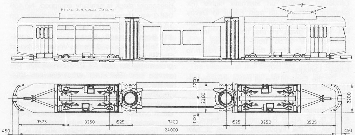
The above drawing, courtesy Schindler Waggon, depicts the 3-unit low floor articulated *Cobra* tram which has been on trial in Zürich since mid-March.
