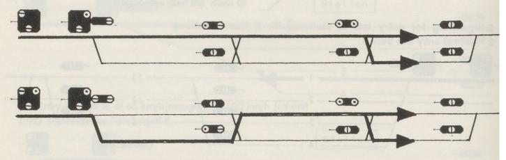
3.4 Entry into an occupied second track section.
