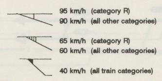
2. Signalling for entry into a station with 2 track sections.
