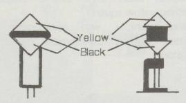
The Senksignal can also be seen as a light signal. It carries a triangular plate, and is in its unlit state, without meaning. It can be used in the circumstances c) or d), above.
