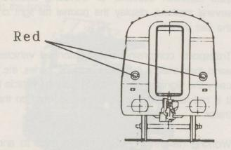
On vehicles with built-in lights, the end of the train is marked by two red lights at the same height, or with one red light to the right.
