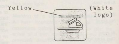
An orange brake show warning board indicates that the vehicle carrying it is prevented from movement by brake shoes (scotches).
