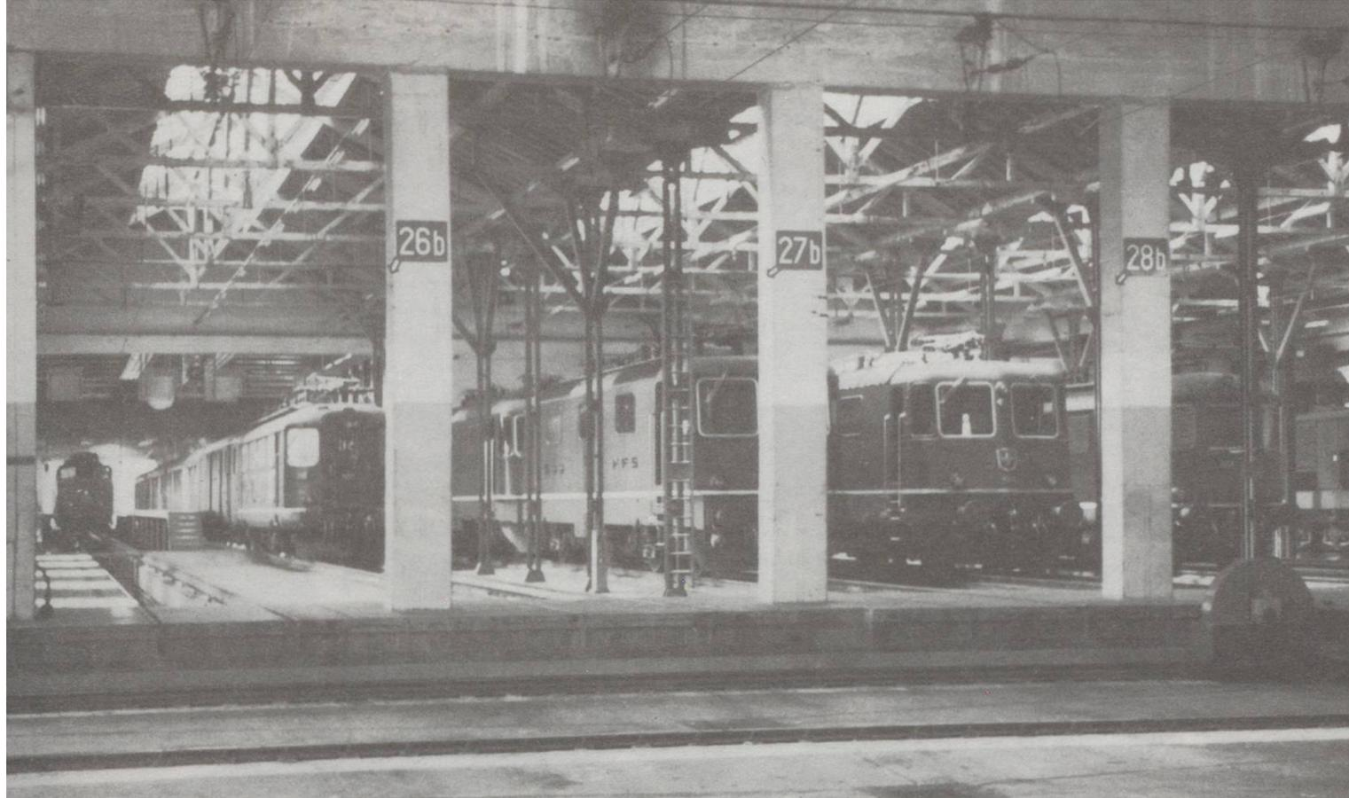
*Inside Lausanne Depot 26 July 1990. Note the traverser tracks in the foreground and both types of Re4/4<sup>t</sup>*
