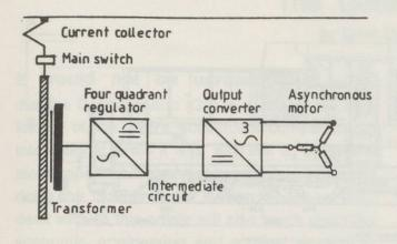
Figure 1 Schematic diagram of converter loco.
