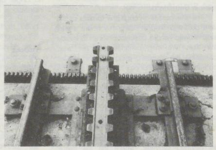
prevent the toothed wheel on the rack from lifting off on the steeper sections, but also centre the vehicle on the track. This means that the outer wheels on the coaches and locos and the rails on which they run merely stabilise the vehicle. I hope that the photo gives you some idea of how they work.
