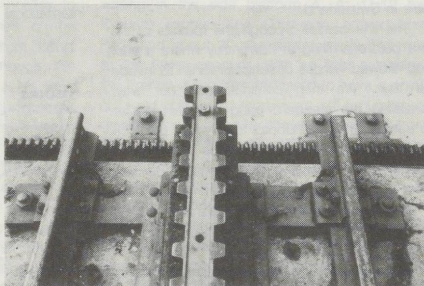
prevent the toothed wheel on the rack from lifting off on the steeper sections, but also centre the vehicle on the track. This means that the outer wheels on the coaches and locos and the rails on which they run merely stabilise the vehicle. I hope that the photo gives you some idea of how they work.
