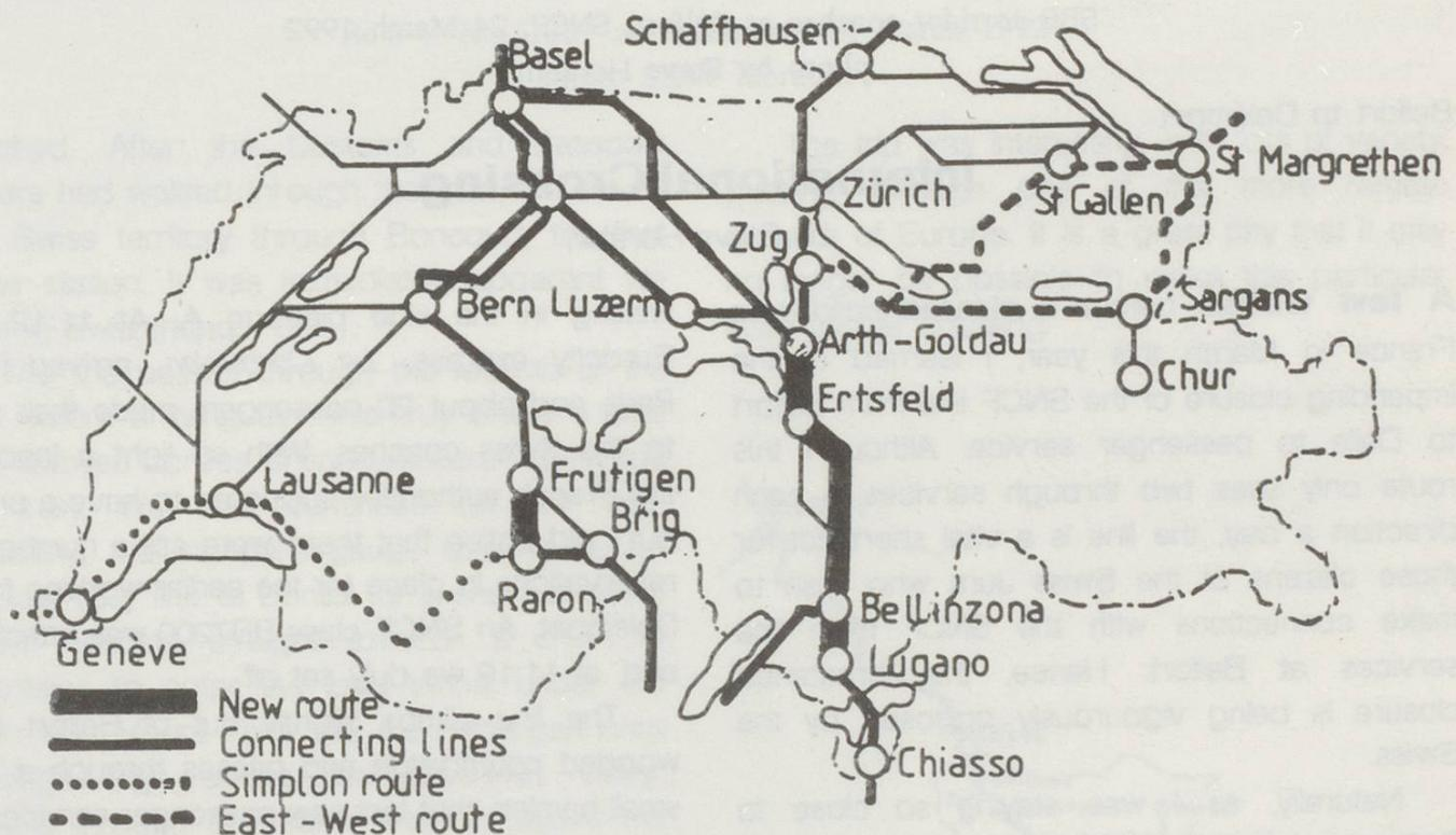
The sketch map above is derived from one which appears in issue 2/92 of the SBB Magazin, showing, diagrammatically, the various routes that will be upgraded in connection with the new deep level basis tunnels under the Gotthard and Lötschberg. Our map in the September 1990 issue of Swiss Express gives rather more detail of the proposed tunnels.
