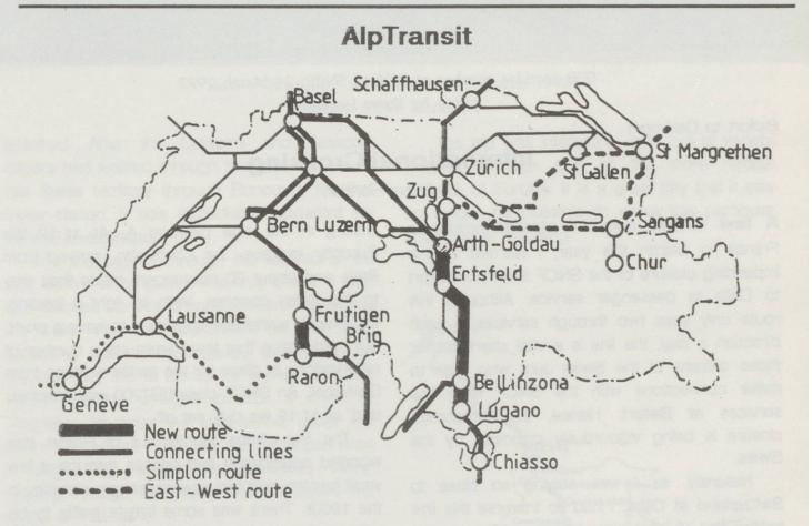
The sketch map above is derived from one which appears in issue 2/92 of the SBB Magazin, showing, diagramatically, the various routes that will be upgraded in connection with the new deep level basis tunnels under the Gotthard and Lötschberg. Our map in the September 1990 issue of Swiss Express gives rather more detail of the proposed tunnels.
