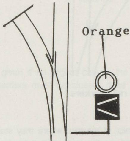
If the point is provided with a fixed lantern with moveable shades, then an additional lantern is required, showing a white edged orange board by day and an orange light by night. The indicator is fixed, irrespective of the position of the point.
