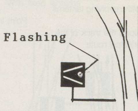
Trains must stop before a Ruckfallweiche displaying a flashing or unlit point indicator.
