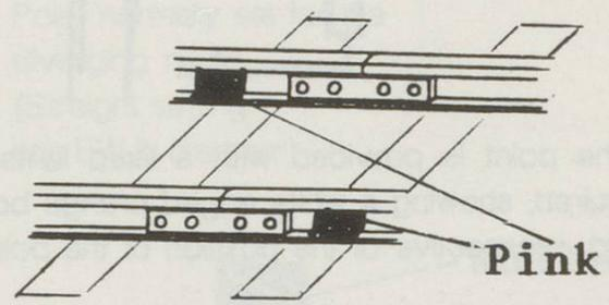
Where local circumstances demand it, the isolated rail section is additionally marked by a yellow peg or yellow-painted cable end connector.
