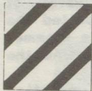
The actual beginning of the restricted section is marked by an **Anfangssignal**, a square white board with three diagonal black stripes.
