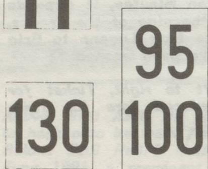
The speed permitted is shown in black on a white board, positioned the braking distance from the start of the speed restriction. If two speeds are shown, one above the other, the higher speed applies to trains of category R (Usually, these days, all passenger trains), while the lower speed applies to all other trains.
