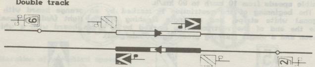
ii) On two-track sections with reversible working, all signals for both directions are positioned on the outer sides of the formation.
