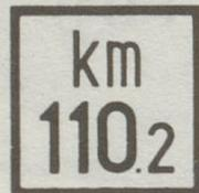
Where the permitted maximum speed of a section changes, the location of the point of change is indicated by a Kilometer marker. Speeds are not marked, these being shown in the working timetable.
