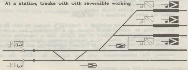
If the restriction is not wholly lifted, a second full set of signals (warning, commencement and end), with with no track magnet, will be placed in position.
