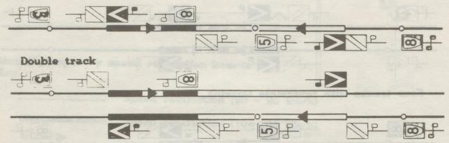
vii) The cancellation signal stands about 50m from the diverging point, or at the clearance point marker. (See future instalment)
