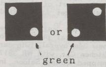
The same size and shape as brake test signals, departure signals are frequently incorporated with them. It is an instruction to the driver, usually by the station staff, that he may depart. It does not override normal running signals, being only an indication that the station work has been completed. The upper light is white, the lower is green and, like the brake test signal, it is double sided .
