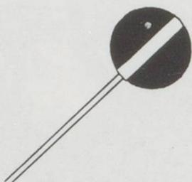
Portable STOP signs take the form of a red disc with a white bar by day. At night a red lamp is hung from the disc.
