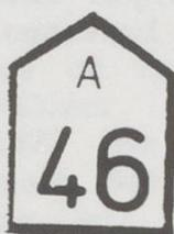
At some locations marker boards, showing either a number of axles or a train length, indicate where the front of a train corresponding to the indicated length should be halted. Longer trains, or trains with more than one locomotive, may pass the board by the length by which the train exceeds the indicated length, whilst shorter trains stop before reaching the board. A series of boards carrying different lengths simplifies the process.
