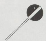
Portable STOP signs take the form of a red disc with a white bar by day. At night a red lamp is hung from the disc.
