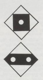
At unstaffed halts, a passenger operated flashing light is located at the braking distance from the halt. The original type consists of a single white light with a square black surround on a larger white diamond-shaped background whilst the later type (GFM and others) has two alternately flashing white lights on a black bar on a white diamond.
