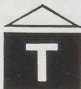
Stations without Transit signals or block posts may be provided with a telephone call signal. Similar to the electric lamp of a Transit signal, these signals carry a white triangular indicator. A flashing T instructs train personnel to use the nearby signal telephone.
