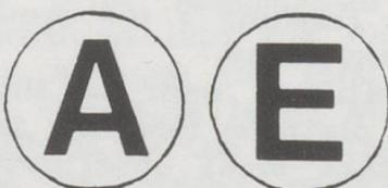
The beginning of a rack section is preceded at a distance of about 150m by a square white board with black numerals, giving the speed allowed on that section. The beginning of the rack rail is marked by a round white board with a black letter A (C in French-speaking areas), and the end of the rack rail by a similar board with the letter E (F in French). The two indications are usually on opposite sides of the same post.
