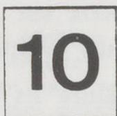
The beginning of a rack section is preceded at a distance of about 150m by a square white board with black numerals, giving the speed allowed on that section. The beginning of the rack rail is marked by a round white board with a black letter A (C in French-speaking areas), and the end of the rack rail by a similar board with the letter E (F in French).
