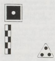
The correct functioning of automatic level crossing equipment is indicated by an orange flashing light positioned at braking distance from the crossing. A black/white chequer board assists identification of the signal.
