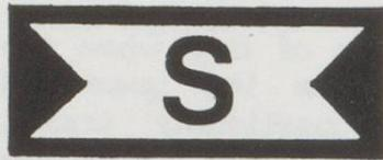
a) if the train magnet (manufactured by Signum) is positioned more than 50m from its associated signal. Some railways (eg BOB) show just M (for Magnet)
