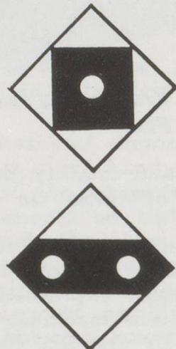
At unstaffed halts, a passenger operated flashing light is located at the braking distance from the halt. The original type consists of a single white light with a square black surround on a larger white diamond-shaped background whilst the later type (GFM and others) has two alternately flashing white lights on a black bar on a white diamond.
