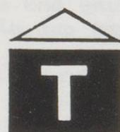
Stations without Transit signals or block posts may be provided with a telephone call signal. Similar to the electric lamp of a Transit signal, these signals carry a white triangular indicator. A flashing T instructs train personnel to use the nearby signal telephone. When unlit, the signal has no meaning ☐
