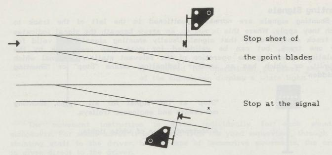
The signal is in the area of the point blades of a single point and is valid for both routes.
