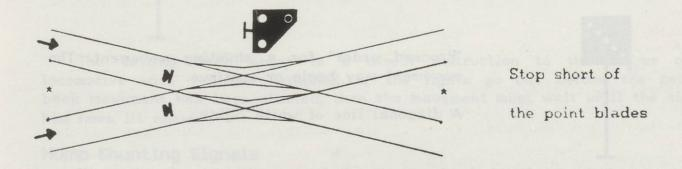
The signal is at the middle of a double slip and is valid for both routes into and away from the double slip.
