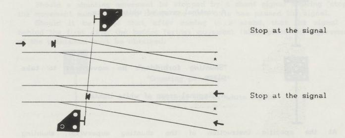
The signal is between the point crossing and the clearance marker of a single point and is valid for only one of the routes.
