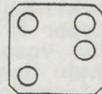
At some stations where the driver's view of the departure signal is obscured, a Weiderholungssignal has been installed which informs the driver whether the departure signal is showing clear or stop. The top two (horizontal) lights, when illuminated, mean that the departure signal is showing stop, the lower two (diagonal) indicate clear.
