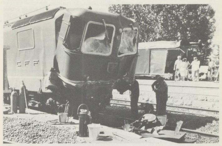
Re4/411 locomotive No. 11343, showing damage to front area.
