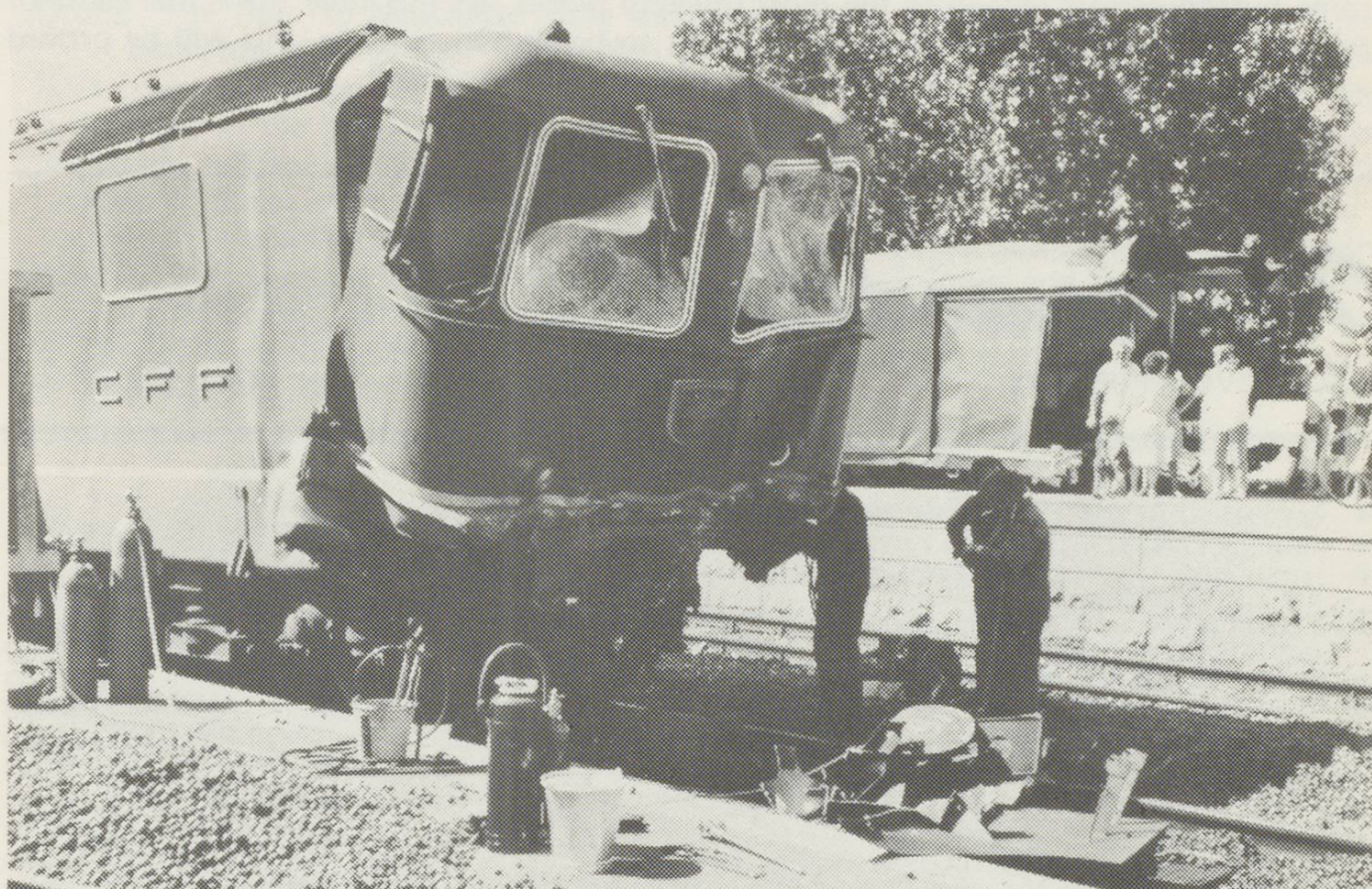
Re4/4II locomotive No. 11343, showing damage to front area.
