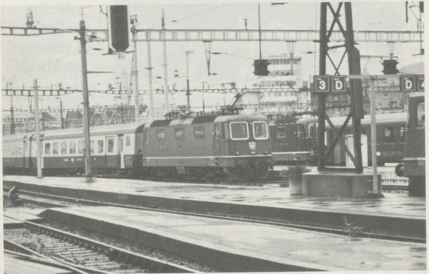
Re4/4II arrives in Zürich with the rebuilt Swiss Express stock on the new Luzern/Zürich Pendlezug service
