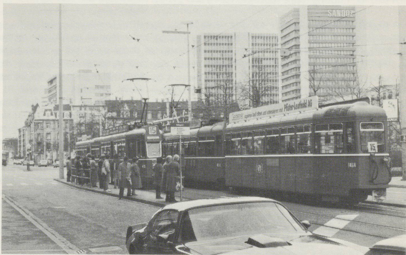
Tram type Be4/4 and B4/4 trailer.
