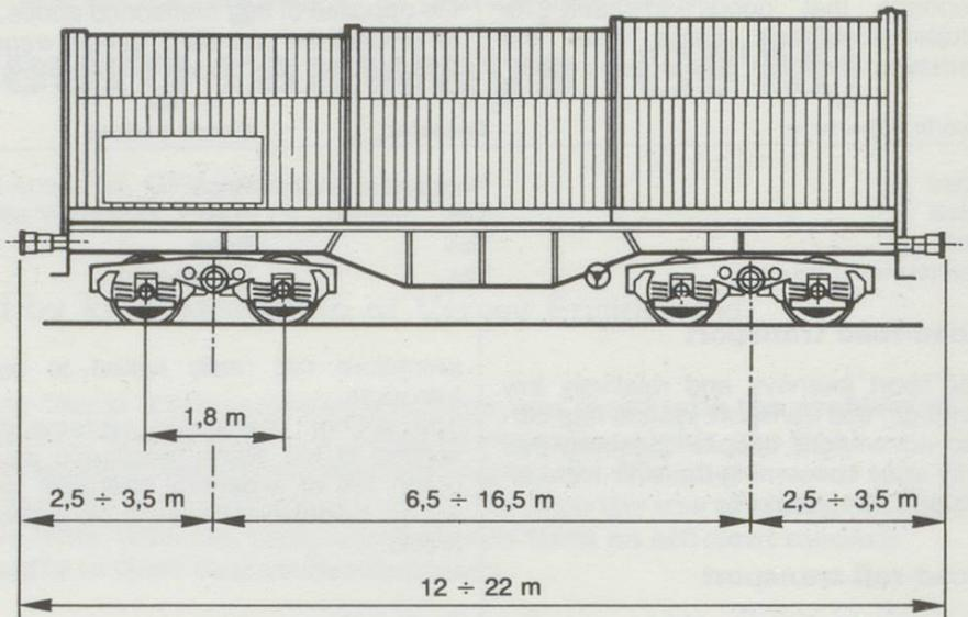
Fig. 3. SG 4-axle wagons with 20 t per axle.
