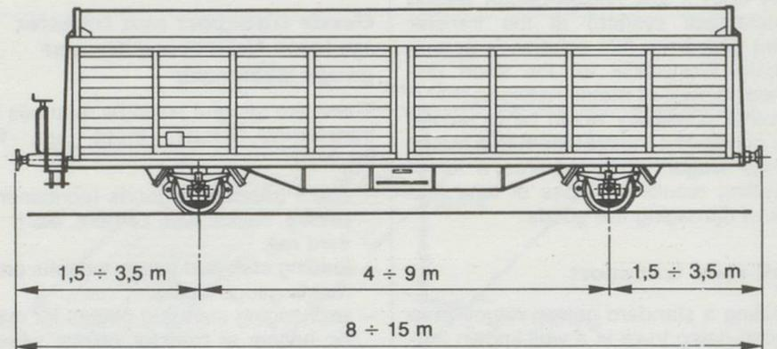
Fig. 4. SG 2-axle wagons with 20 t per axle.
