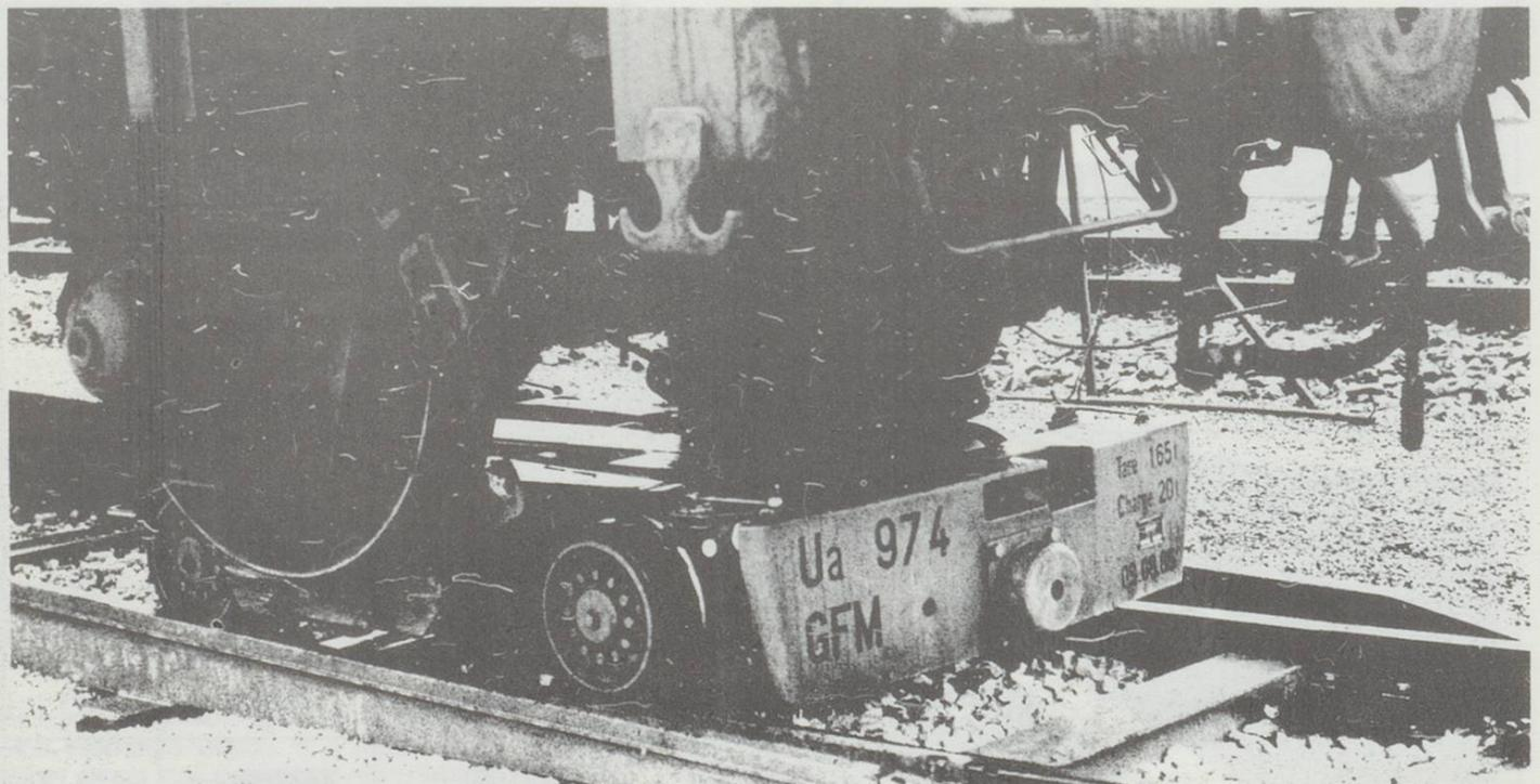
Fig. 14. VEVEY transport bogie on GFM network.
