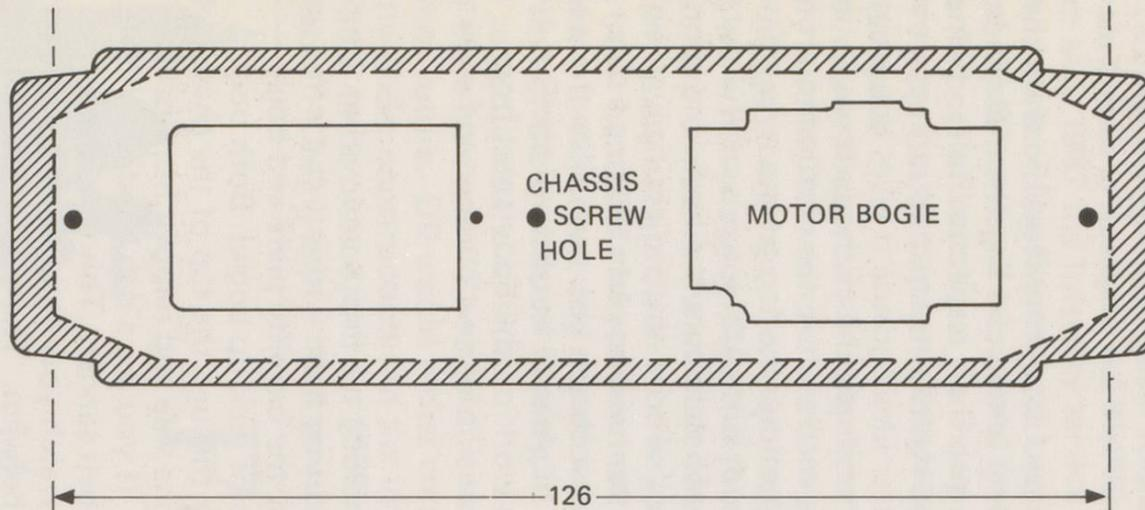
CENTRAL CHASSIS WEIGHT, SHADED AREA TO BE REMOVED, TO CLEAR CENTRAL PILLAR AND CHASSIS MOUNTING SCREW.
