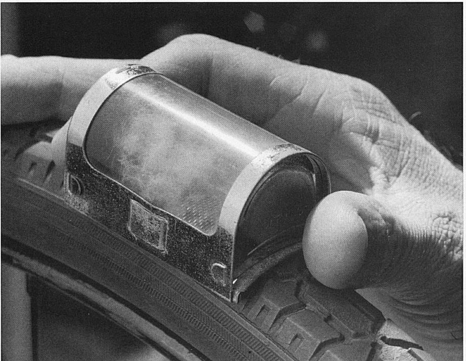
21 An automatic bell. The mechanism is actuated by pulling the string, whereupon the bell runner is pressed on the front wheel and the bell rings till it is withdrawn again or the bicycle comes to a stop.
