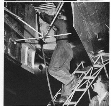
Right: During the short stop of a foreign aircraft at Zurich Airport, the hydraulic equipment of the aeroplane's landing gear is supplied with oil is supplied with oil.
