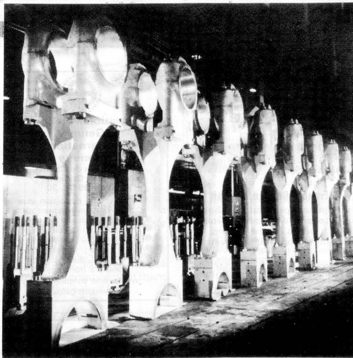
NO, not the winning entry in an architectural competition, but a line of connecting rods for a large Sulzer diesel engine. Each connecting rod is part of a system which transfers 2500 kW (3400 hp) from one cylinder to the main shaft of the engine. This means each connecting rod transfers an output equal to that of a small railway locomotive.
