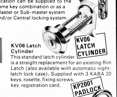
KV06 Latch Cylinder This standard latch cylinder is a straight replacement for an existing Rim Latch (also available with automatic night-latch lock case). Supplied with 3 KABA 20 keys, rosette, fixing screws, key registration card.
