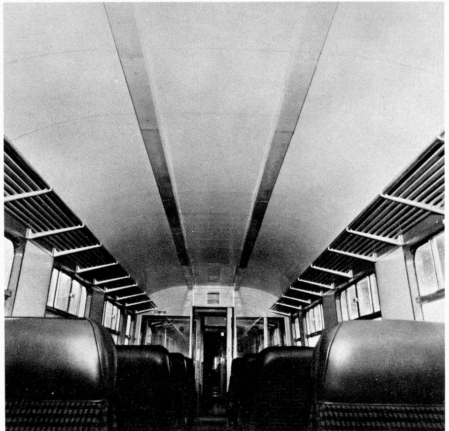
Prototype replacement ceilings made from lightweight composite sandwich are already in use on the Nottingham-Derby-Crewe line. The Kent coast carriages will incorporate very similar ceilings having just the same profile.
