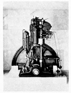
One of the first Sulzer four-stroke diesels. Installed as a pump drive in 1903, it ran ten hours a day until 1951 without giving trouble.
