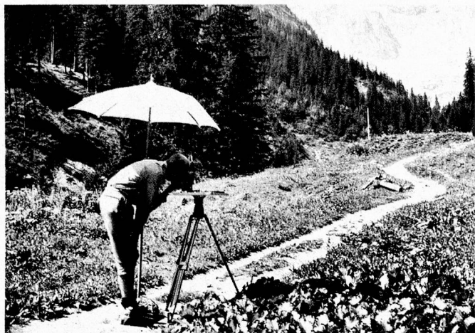
Topographical details were surveyed using the planetable
