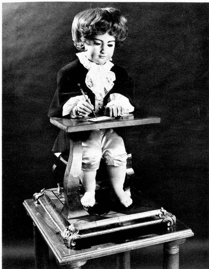
Front view of the "Draftsman", completed in 1774 by Jaquet-Droz father and son, one of the three famous mechanical dolls from the Museum of Art and History in Neuchâtel. Courtesy of SNT0.
