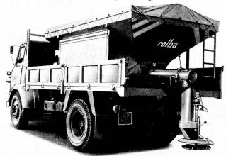
A wide variety of spreading patterns are achieved due to the unique 360° turnable feeding nozzle fitted to all Rolba-Weisser Bulk Gritter Bodies. Standard components are used throughout the range enabling interchangeability of individual parts between different models and every Bulk Gritter unit carries a two-year Guarantee. Smaller attachments are available for tractors, Land-Rovers and individual lorries.
