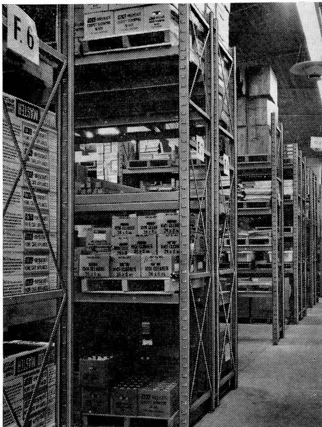
The world's most versatile two-piece racking system, Acrowrak Series 75, the choice of warehousemen, is totally engineered for strength plus safety. Complete systems or simple rack installations match customer needs for any particular handling problem. High-speed assembly and dismantling for re-use are matched by impressive economy. Upright frames and shelf beams lock firmly in a range of sizes for numerous applications — Acrowrak Series 75 can solve your storage problem.
