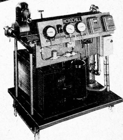
Acrochill offers this typical performance: 300 gph with water discharged at 60°F with a temperature difference of 10°F. This machine is widely used in injection moulding, metal plating, bakery and confectionery. All units are factory-tested for rapid installation.
