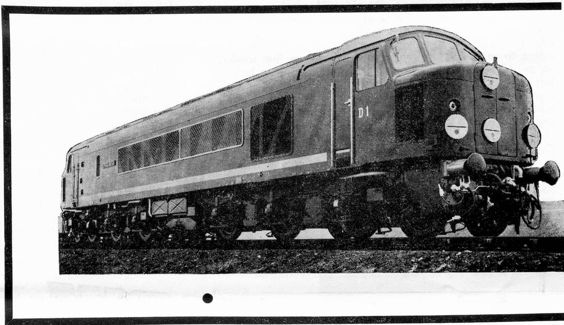
603 Sulzer engines with ratings of 1160 to 2500 h.p. are being supplied for British Railways diesel locomotives. Of these over 200 are now in service.
