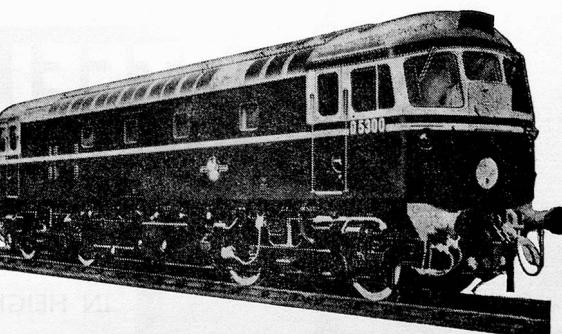
B.R.W.C. type 2 locomotive fitted with the 6LDA28 engine.
