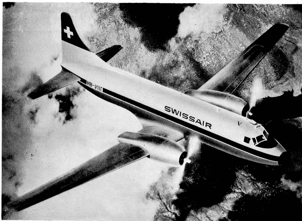
Soon to join Swissair's fleet: the new Convair "Metropolitan". Note the black-painted nose housing the weather-mapping radar.
