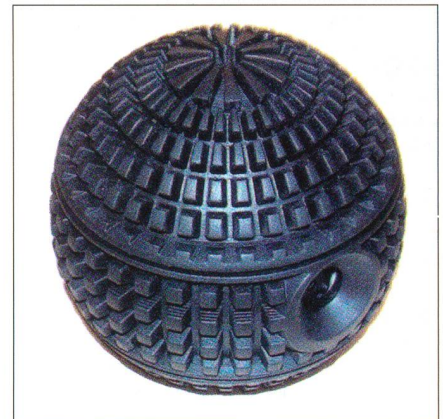
Short Range Throwing Camera von Defence Optical Systems
