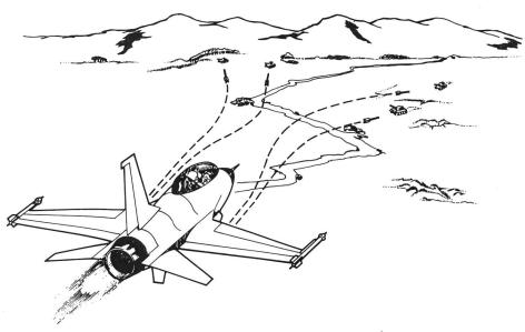
BUSTING TANKS WITH HVMs -- This sketch shows an F-16 aircraft launching several Lockheed-built hypervelocity missiles (four are shown for simplicity). The missiles are laser-guided and independently targeted.
